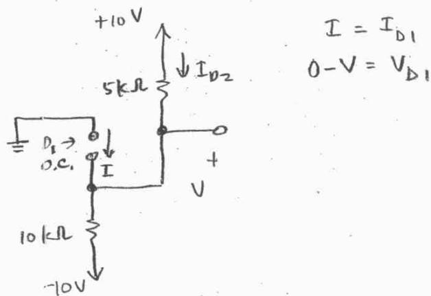
$$I_{D2} = \frac{10 - (-10)}{(10 + 5) k} = \frac{4}{3} \text{ mA} ; V_{D2} = 0 \text{ since S.C.}$$
