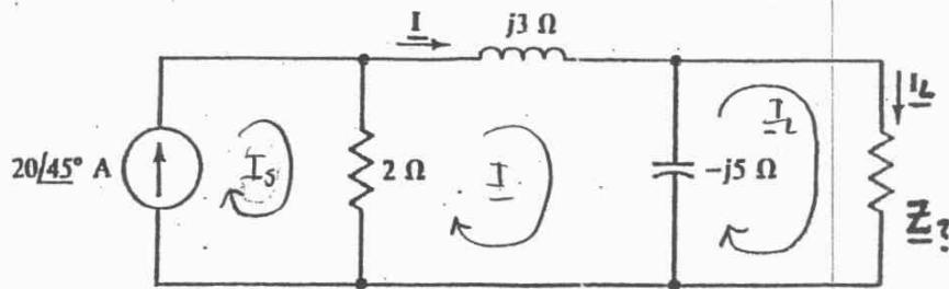
$$I_S = 20 \angle 45^\circ \quad I_L = 6.85 \angle -7^\circ$$
