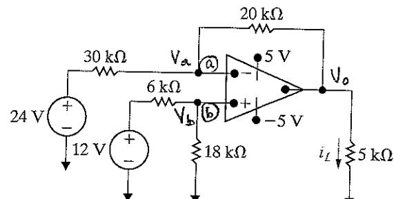
2. 5.9  $-5 < V_o < 5$  for  $0 < V_g < 5 \text{ V}$ . Note  $V_a = 2.5 \text{ V}$ .
