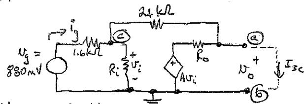
(b) What is output resistance? Find by applying  $V_{test}, I_{test}$  @ output -- equiv to Thevenin res.
