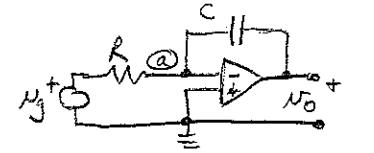
$$\sum i = 0 = \frac{v_g - 0}{R} + C \frac{d}{dt}(N_0 - 0) \Rightarrow \frac{dv_0}{dt} = -\frac{1}{RC} v_g \Rightarrow v_0 = -\frac{1}{RC} \int_{-\infty}^t v_g(t') dt' ; \frac{1}{RC} = \frac{1}{10^3(800)(10^{-12})} = 1.25 \text{eV}$$
